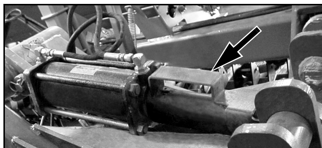
Figure 34 Cylinder Lock Channels Inserted for Transport - Front Box Cylinder Shown
