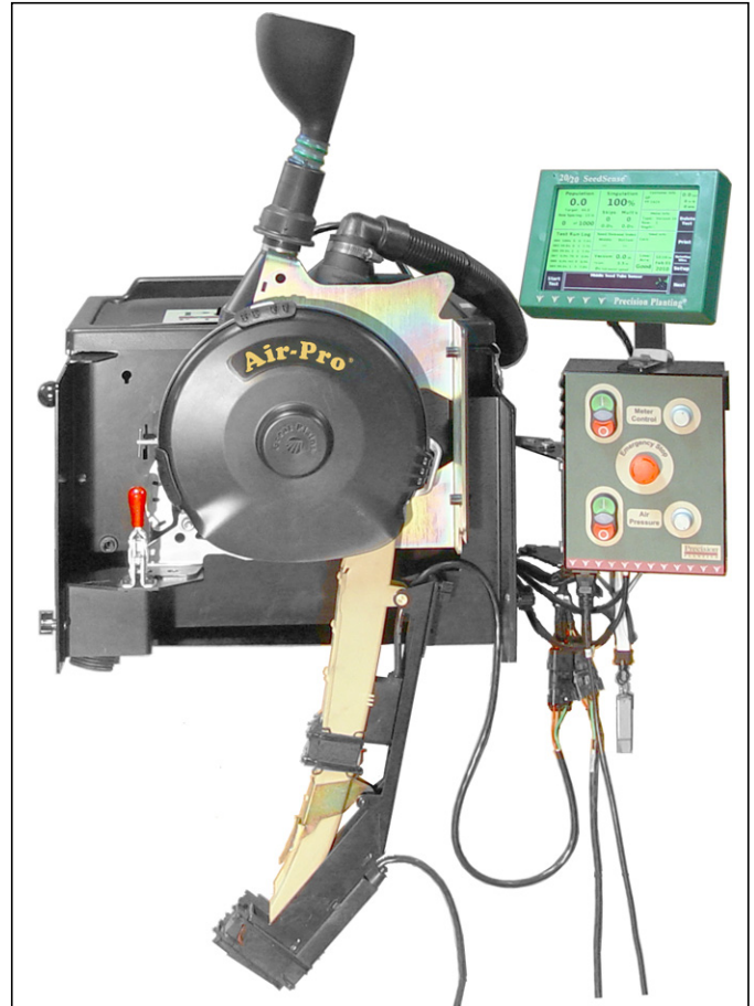
Figure 1 Air-Pro® Meter Mounted on the MeterMax® Ultra Test Stand
