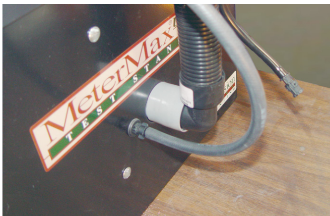
Figure 9 Hoses Connected Back of Stand
