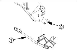
Route blade separator's attached fertilizer tube through opener shield and attach elbow cap. Route tubing from aligned wetboom port down to the blade separator's elbow cap.
