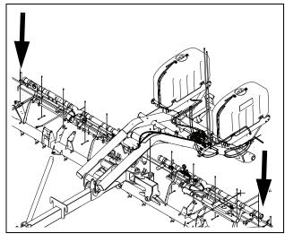
Split short Accushot seed sensors into two even piles. Install all of one set of seed sensors onto the rows starting from the first available opener on the left-side of the machine. Then install the remaining seed sensors onto the rows starting from the first available opener on the right-side of the machine.
