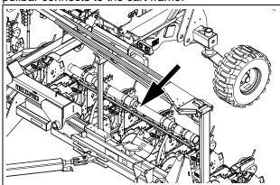
On the left-hand side of the pullbar, install the control box mount onto the implement frame using four sets of bolts, washers, lock washers, and nuts.
