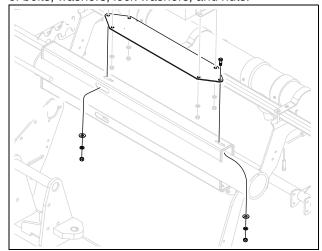
Install control box onto the control box mount using four sets of bolts, washers, and nuts.
