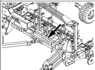
On the left-hand side of the pullbar, install the control box mounts onto the implement frame using four sets of bolts, washers, lock washers, and nuts.
