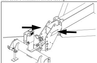
Locate the frame on the left-hand side of the machine. Install remaining Accushot controller decal to frame.
