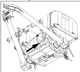
If no holes are present for pump in the cart frame, you will need to make them with a standard power drill. Measure holes so they are 8" apart. Make sure hole markings align with pump mount holes. Drill holes using a 0.44" drill bit.
