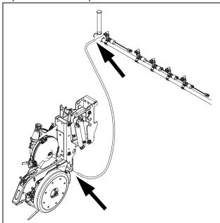
Secure fertilizer tube to the opener using supplied zip ties.
