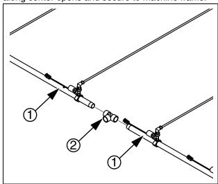
Route Accushot valve harness along center. Connect harness ports to controller.
