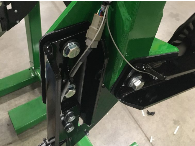
Secure EC wiring harness to terminal bolts on front coulter discs and rear runners.
