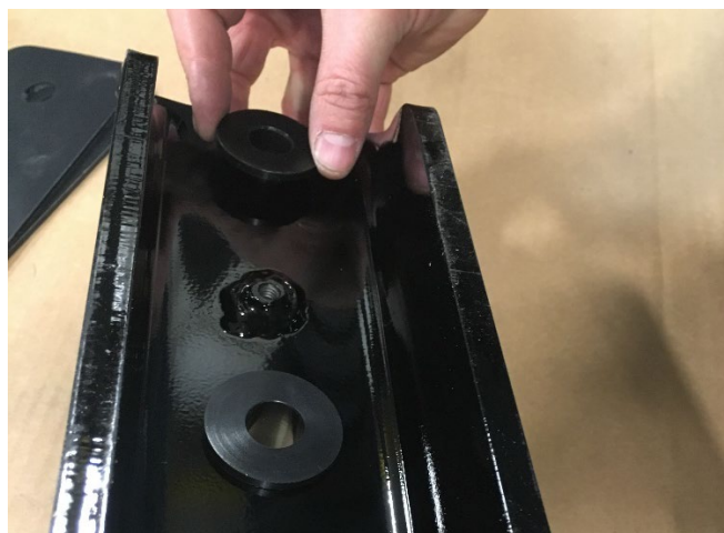
If arms have been removed, ensure plastic bushings are inserted before installing.
