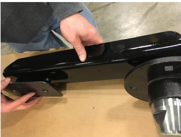
Also, ensure plastic insulator is installed between arm and mount.
