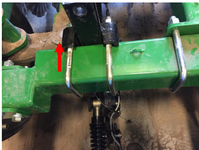
Install coulter clamps with coulter clamps exactly aligned with marked arrows.
