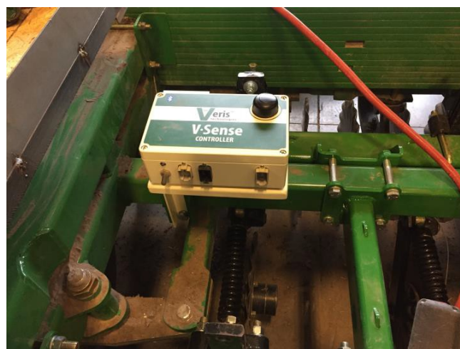
Install VSENSE and run cabling for communication and 12V power.
