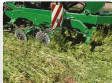
The Turbo Coulters facilitates drilling into high volumes of residue
