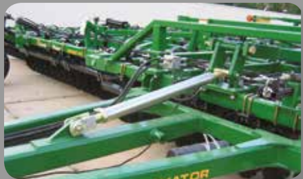
SELF-LEVELING HITCH - The Disc-O-Vator features a clean, slim profile, self-leveling hitch design with turnbuckle height leveling adjustment.
