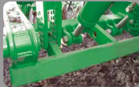
DEPTH CONTROL - Positive depth control is a standard feature on 23C Series wide folding machines.
