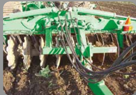
REAR DRAWBAR AS STANDARD - A rear drawbar, standard on 2B and 23C models, allows a DD Ring press to be towed for reconsolidation.
