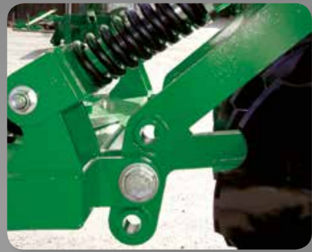
ADVANCED GEOMETRY - The drawbar is pulled from the disc axle allowing the disc angle to be altered on the move without upsetting the stability, balance and tracking of the machine.
