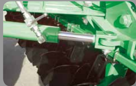
HYDRAULIC GANG ANGLING - Hydraulic gang angling is only required on the front gang due to the innovative frame design.
